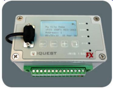
The iRIS 150FX is a small, compact datalogger featuring an LCD display and keypad. It can be connected to a wide variety of sensors, and features two analogue (0-5V, 0-20mA) inputs, two digital inputs, SDI-12 serial instrument support and a single digital output for alarm or control purposes.
